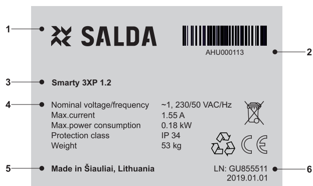
1 - Logo; 2 - Product code (SKU); 3 - Product name; 4 - Technical data; 5 - Production place; 6 - Lot number and production date.
